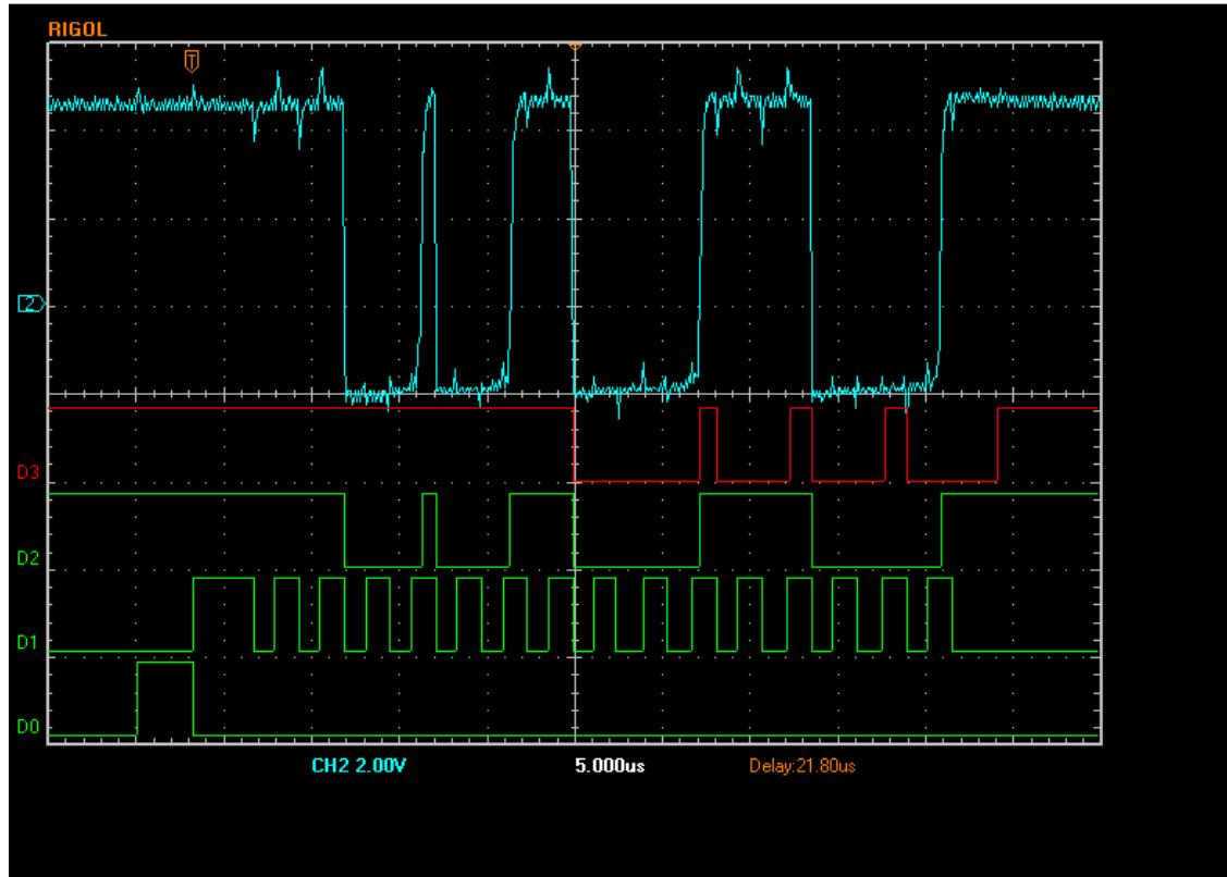
The bottom trace is the convert line, the line above the clock line. D2 is the magnitude data and D3 is phase, present still but the code is ignoring it. The top trace is a scope rather than a logic analyser trace on the ADC data out line. More of this later. In the trace can be seen the convert line go high followed by the clock line high whih then goes low 16 times, one for each bit. The data can be seen clocking out above this as D2.
