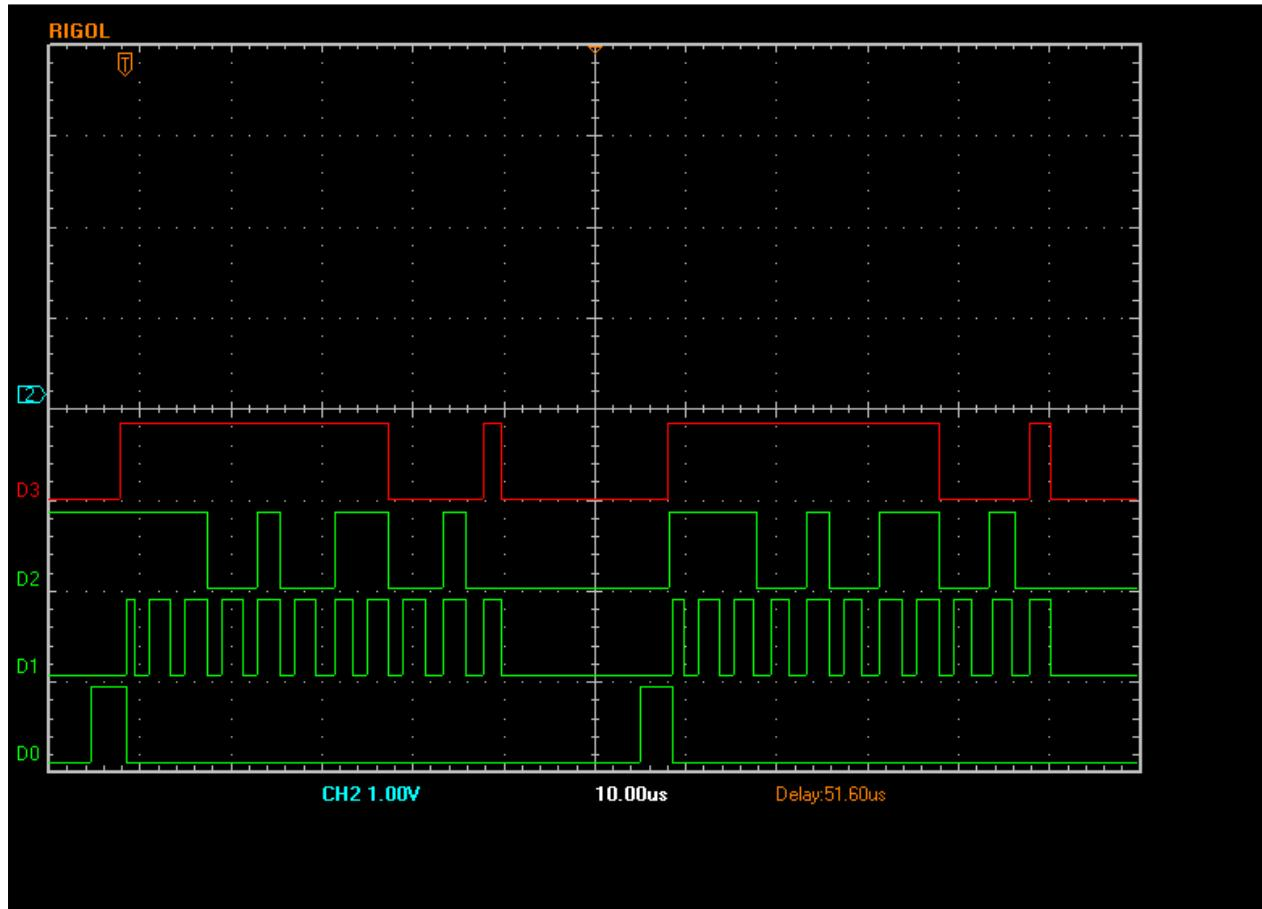
The trace starts with a convert signal, followed by an extra clock edge that the lt1865 apparently needs followed by 10 falling edges. It is not quite as the datasheet but follows the basic code so some testing may be needed (I don't have an LT1865 to try).
