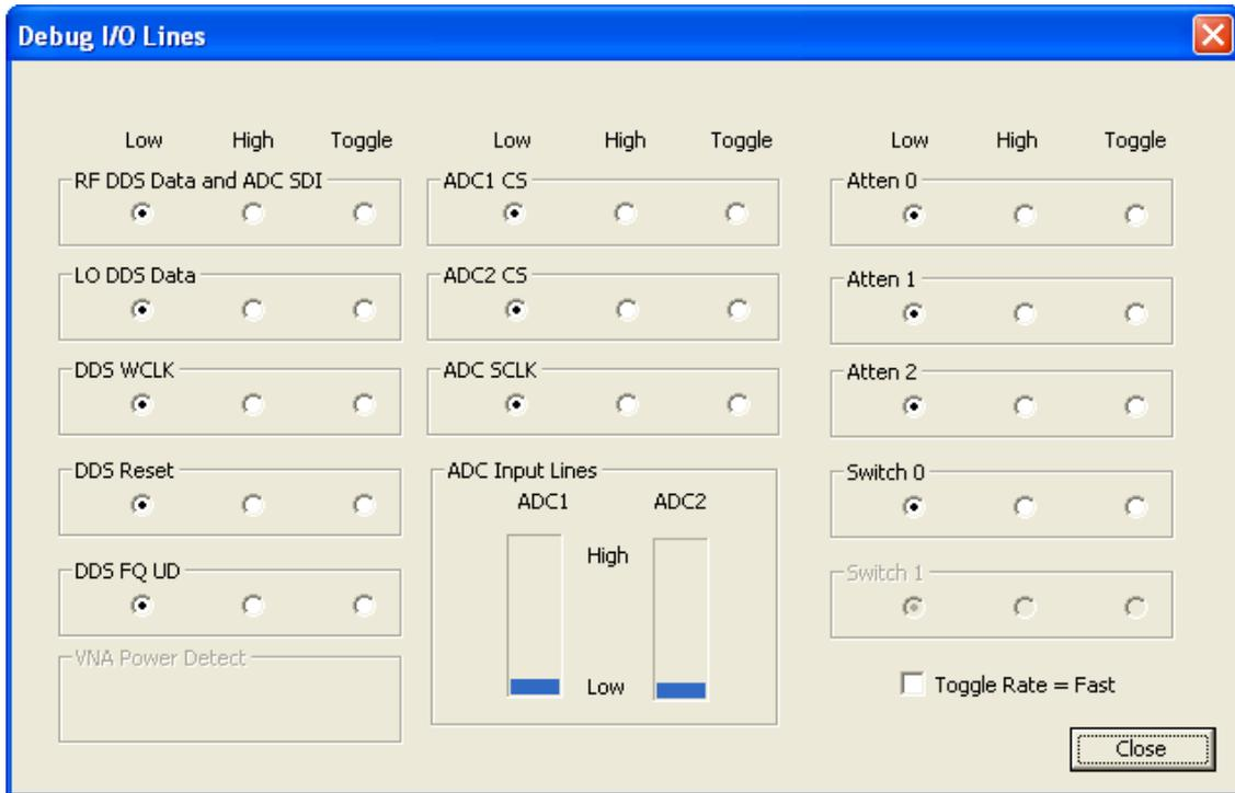
Each I/O line may be set low, high or to toggle. Connect a meter to the parallel port output and see if this is the case for each line. Alternatively, each may also be set to toggle at a fast (30 times / second ) or slow ( twice per second ) rate.
