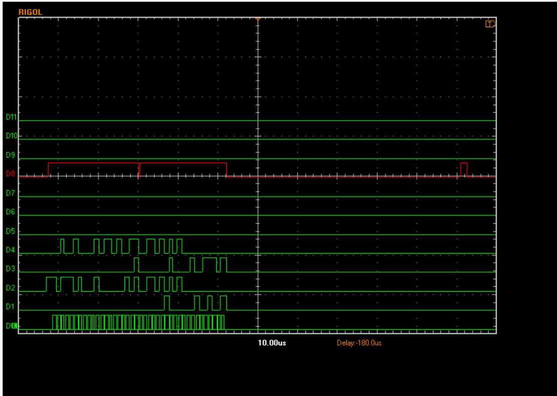
Ignore the transient in the middle of the signal high of D8 – this is an analyser glitch. The data lines are set, the SLIM-CB latch line raised and the data is clocked out into the devices. When it is over, the latch line is lowered, and raised again briefly 60 usec later to latch filterbank.
