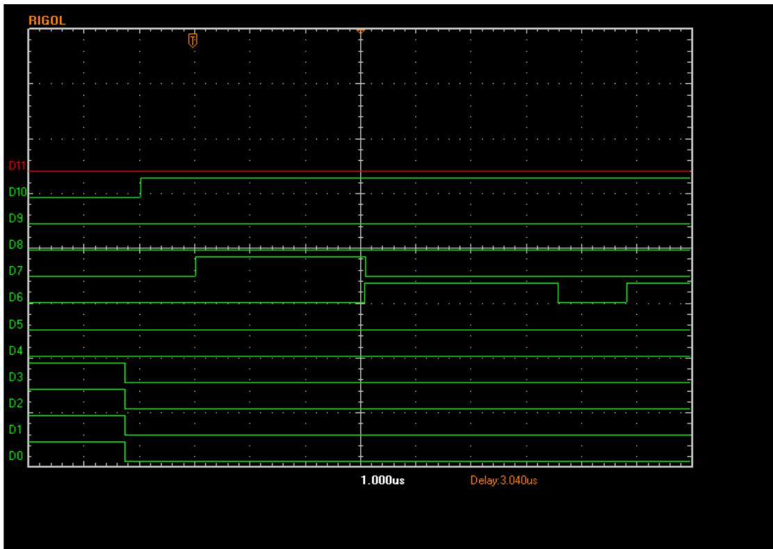
The bus is forced low (D0-7). D10 is then raised (AUTO, opening the P3 latches and giving write access to ADConv and ADSerClk). 1us later, ADConv is raised (D7) and
