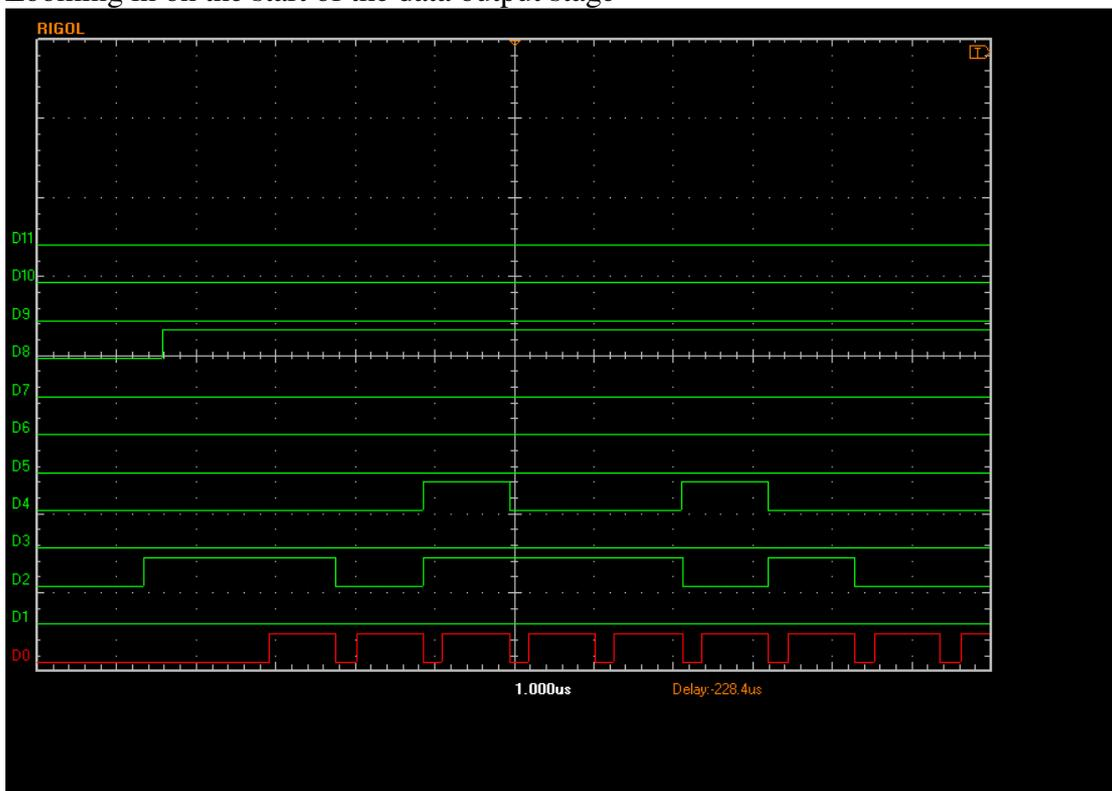
The clocking cycle for the data is just over 1usec per bit, and there are 40 bits that are clocked. At the end of the 40 bits (below) the latch line is lowered again.
