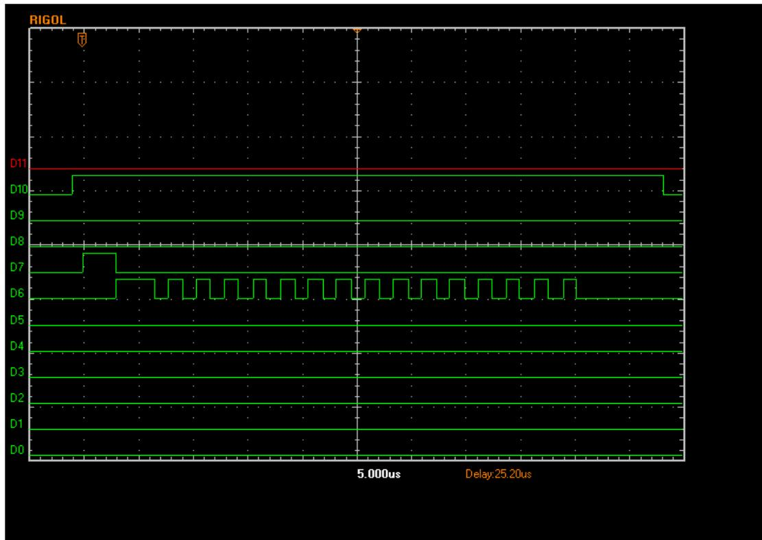
The data bus is set to zeros, then D10 is raised. You can't see the bus being cleared so here the low 4 bits of the bus have been forced high before the convert function is called
