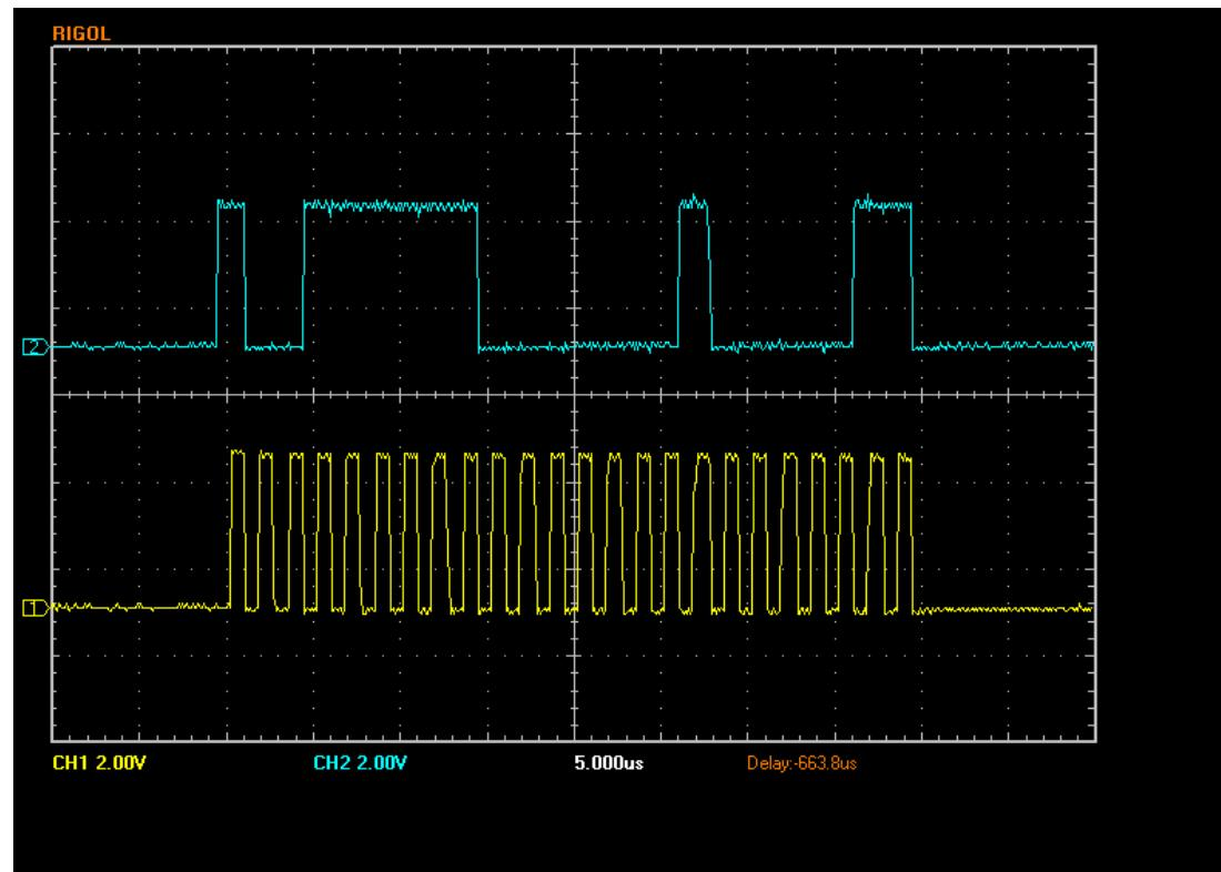
Zooming in on the first 2 bits...the clock duty cycle is 800 nsec low / 800 high
