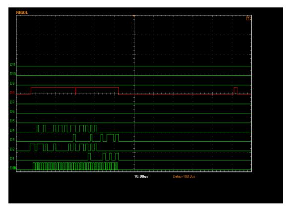
Ignore the transient in the middle of the signal high of D8 – this is an analyser glitch. The data lines are set, the SLIM-CB latch line raised and the data is clocked out into the devices. When it is over, the latch line is lowered, and raised again briefly 60 usec later to latch filtbank.
