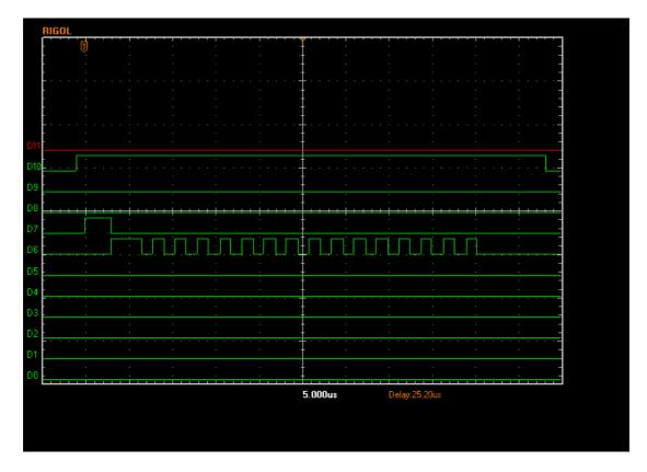
The data bus is set to zeros, then D10 is raised. You can't see the bus being cleared so here the low 4 bits of the bus have been forced high before the convert function is called
