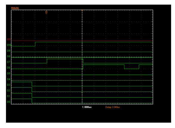
The bus is forced low (D0-7). D10 is then raised (AUTO, opening the P3 latches and giving write access to ADConv and ADSerClk). 1us later, ADConv is raised (D7) and
