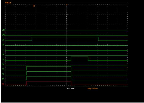
The data lines are set and the latch line raised, which latches data into the DDS and PLL chips. Then pdm data is latched by D5 and the bus latch closed again
