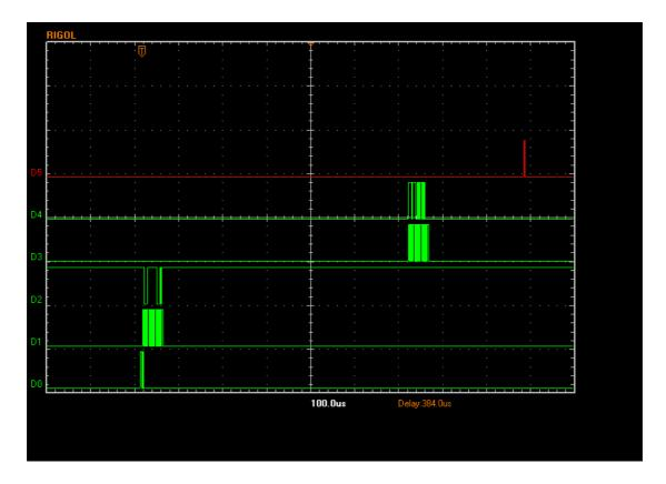
From the perspective of the PC, the time taken to set the DDS is irrelevant as long as it is reasonably fast as this is being handled in parallel to the main PC program running. The only critical timing is the delay from when we ask the ADC to convert (some time prior to the actual conversion above depending on USB framing – anything from 0 to 125 usec) to when it gets the result (probably about 125 usec after the conversion is complete).
